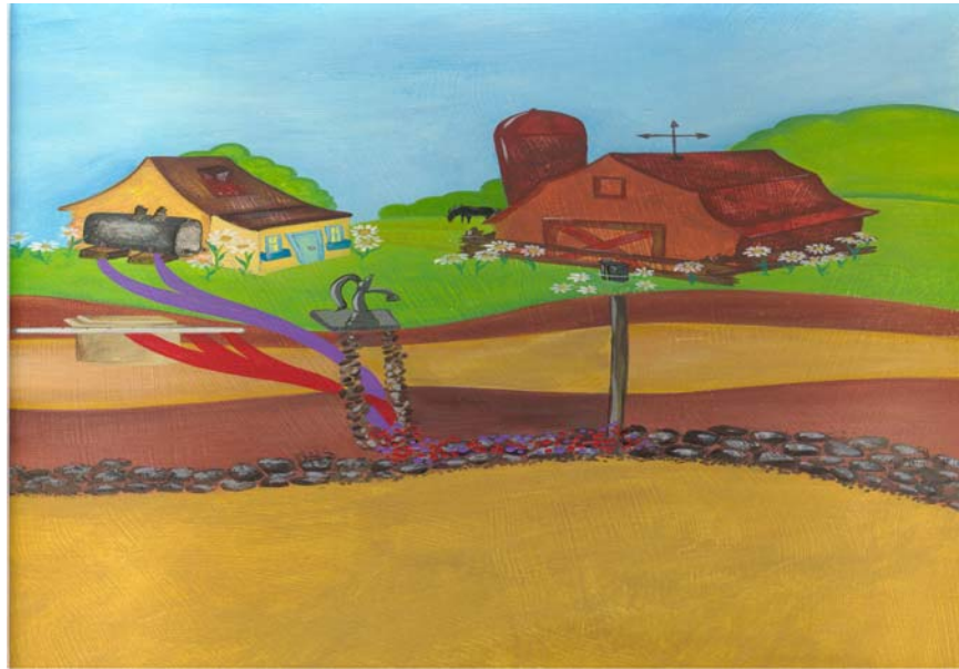
Figure 9.1 Fieldstone Lined Well Receiving Contaminants
